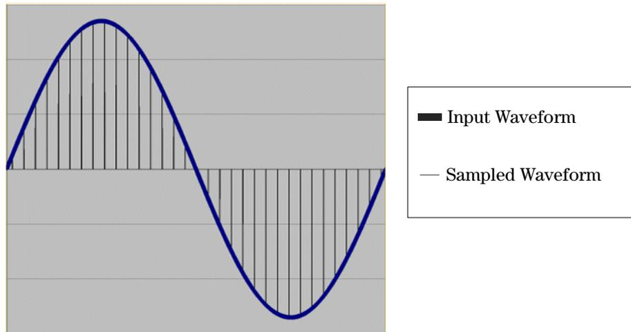
Figure 4.4 Input & Sampled Waveforms
