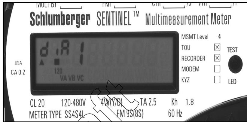
Figure 6.3 Example of Diagnostic #1 Error Display
