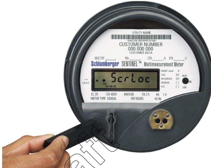
Figure 3.3 Activating the Magnetic Switch
